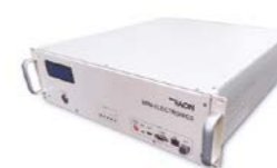
BPM Controller for RAON Accelerator • 16 RF inputs and 4 BPM processors per controller • Position and phase resolution better than 5 μm and 0.1° • Embedded EPICS IOC and Channel Access
