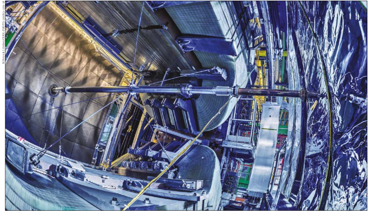
Rhapsody in blue LHCb's dipole magnet sorts particles that are boosted in the forward direction (from right to left), near the beam pipe.
